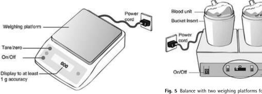
Fig. 4 Laboratory scale for weighing components
