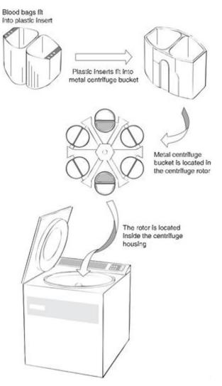
Fig. 3 Centrifuge insert, bucket and rotor
