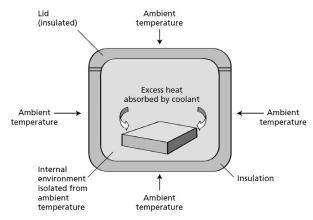
Figure 2 Temperature-controlled blood and component transport container
