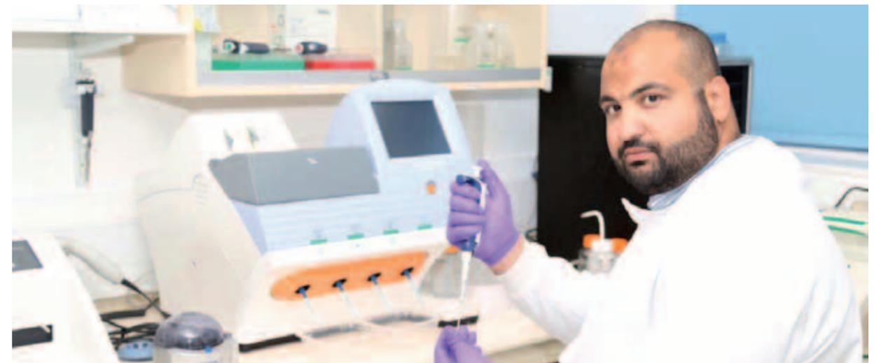
*The last step on next generation sequencing which is loading to chip with the sequencing reaction and the photo shows that Ion Torrent Personal Genome Machine.*
